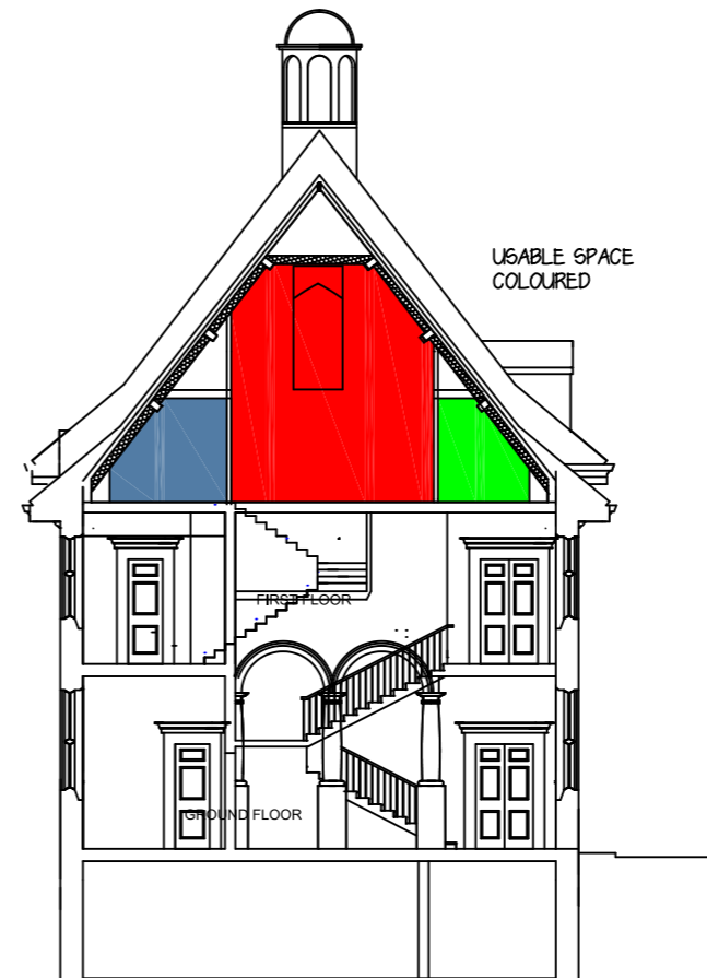
SECTION THROUGH STAIR AND ROOFSPACE
