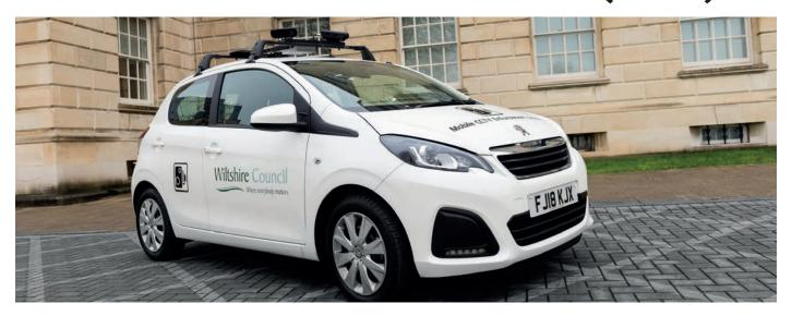
The new MEV has been introduced and is being used tactically for a wide range of traffic management, monitoring and enforcement applications. Linked to the council's virtual permit database, it operates across residential parking zones to detect parked vehicles that do not have valid permits. The vehicle is also equipped to carry out a number of additional activities for greater flexibility.
